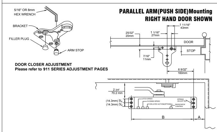
The hand must be determined & changed if necessary before the bracket is mounted to the door stop(top jamb). Refer to page 1.
